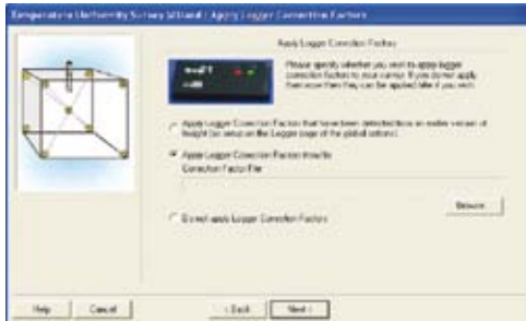
Apply Logger Correction Factors Wizard prompts users to apply mandatory instrument correction factors during setup
